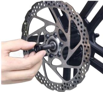
11 Lift the body and align the front fork with the bearing screws on the front wheels
