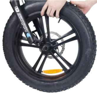
12 Put the front fork on the bearing screw and find the matching nut
