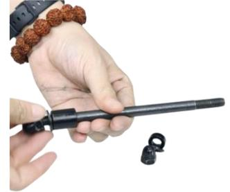
10 Insert the bearing screws into the corresponding holes in the front tire
