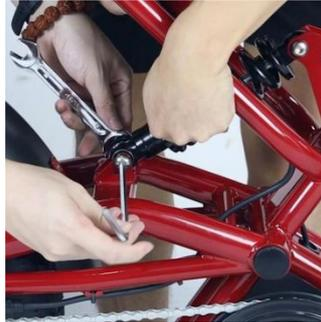
9 Remove the nut from the bearing screw
