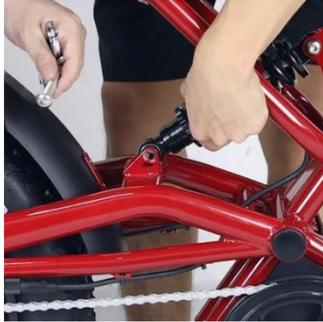
8 Use the tool to install the screws and tighten them
