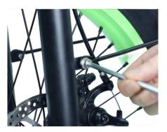
Use a tool to tighten the screws to secure the front fender and headlight into the middle of the front fork
