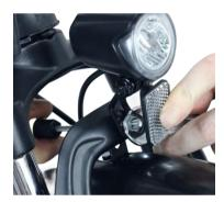
Screw the retaining brackets on both sides of the fender
