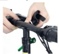
Cover the retaining clasp and tighten the screw
