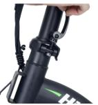
Press the key towards the keyhole and turn the key to the "PUSH" button to remove the battery
